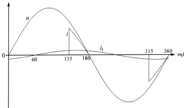
Fig. 2. Voltage and current in circuit shown in Figure 1
