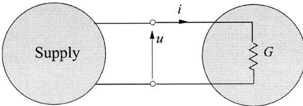
Fig. 9. Single-phase circuit with resistive load
