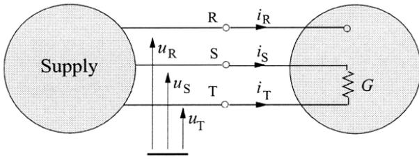
Fig. 7. Three-phase circuit with unbalanced resistive load
