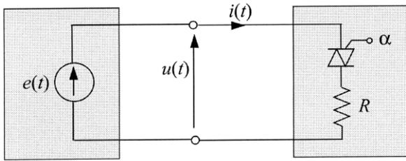
Fig. 1. Circuit with resistive load and TRIAC
