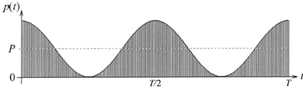
Fig. 8. Instantaneous power variability at supply terminals in circuits shown in Figure 7
