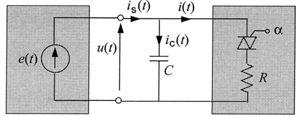
Fig. 3. Resistive load with capacitive compensator of reactive power
