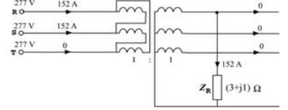
Fig. 10. Example of three-phase system with unbalanced load
