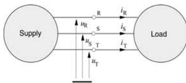
Fig. 1. Three-phase, three-wire system
