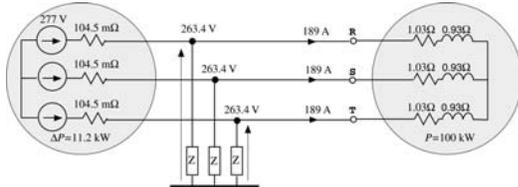
Fig. 6. Balanced load equivalent to unbalanced load in Fig. 6 with respect to power loss in the source
