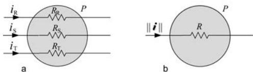
Fig. 3. Three-phase device (a) and its equivalent (b)
