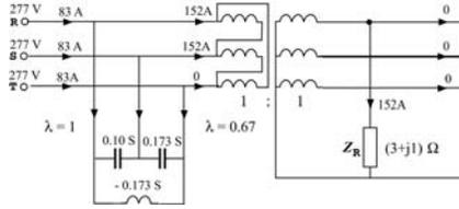
Fig. 12. Unbalanced load with balancing compensator
