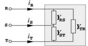
Fig. 8. Equivalent load in  $\Delta$  structure
