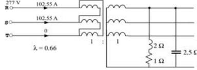
Fig. 13. Circuit with unbalanced load
