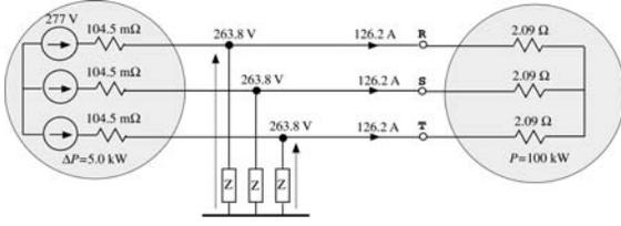
Fig. 4. Circuit with balanced resistive load
