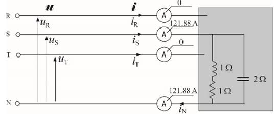
Fig. 7. Example of unbalanced load.
