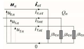
Fig. 5. Reactive load equivalent to the original load with respect to its reactive power  $Q_n$  of the  $n^{\text{th}}$  order harmonic.
