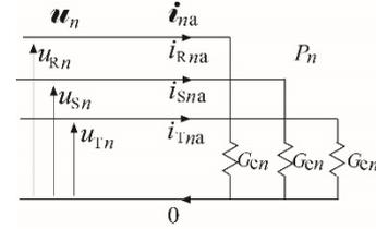
Fig. 4. Resistive load equivalent to the original load with respect to its active power  $P_n$  of the  $n^{\text{th}}$  order harmonic.
