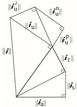
Fig. 6. Diagram of three-phase rms values of CPC.
