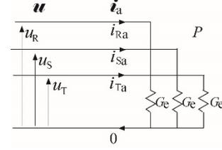
Fig. 3. Resistive balanced load equivalent to the original load with respect to its active power  $P$ .
