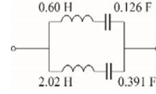
Fig. 6. Structure and parameters of a compensator branch.
