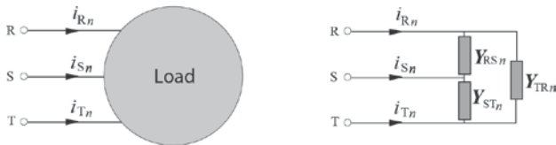
Fig. 13. A load and its equivalent circuit in \Delta configuration for the n^{\text{th}} order harmonic.
